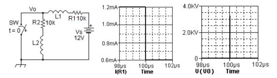
The magnitude of the voltage is over 3000 V and the duration is very short. This is because inductors oppose a change of current. L2 acts like an open circuit initially, so that L1 is discharging into a very high resistance, which means a very short discharge time constant and large voltage amplitude. This impulse may be modeled by the Dirac delta function.
