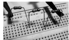
R<sub>TS</sub> = \_\_\_\_\_ (measured total series resistance)
