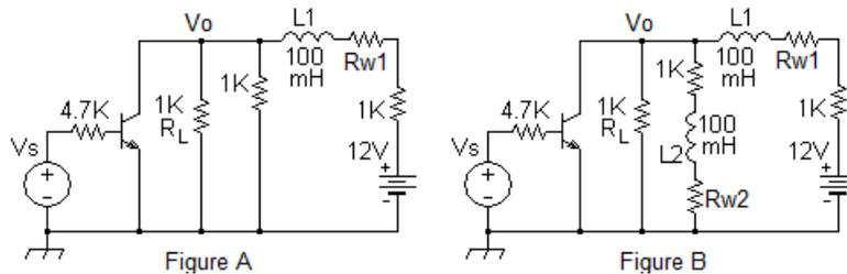
3. Connect channel 1 of the oscilloscope to the function generator and channel 2 to measure  $V_o$ . Trigger on channel 1.
