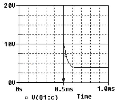
8. Expand the oscilloscope display by adjusting the volts per division, time per division, and trigger controls to most accurately measure the peak amplitude of the positive pulse,  $V_P$ , its decay time constant,  $\tau$ , and steady state voltage,  $V_{SS}$ .
