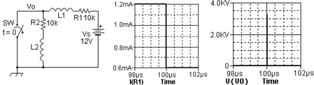
The magnitude of the voltage is over 3000 V and the duration is very short. This is because inductors oppose a change of current.  $L_2$  acts like an open circuit initially, so that  $L_1$  is discharging into a very high resistance, which means a very short discharge time constant and large voltage amplitude. This impulse may be modeled by the Dirac delta function.
